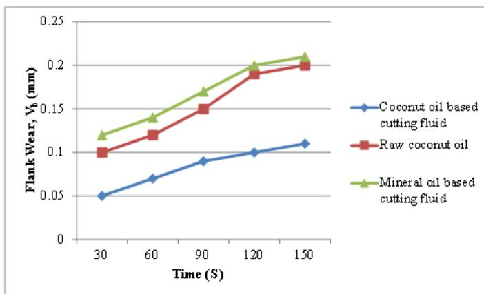
coconut oil-based cutting fluid was established further by the results of the tool life test. The tool wear was the least during the application of coconut oil-based cutting fluid during the whole length of the tool life test (Figure 10). Moreover, SEM photographs (Figure 11 (a), (b), and (c)) of worn inserts indicated less damage to the cutting edge when coconut oil-based cutting fluid raw coconut oil and mineral oil-based cutting fluid were used.
